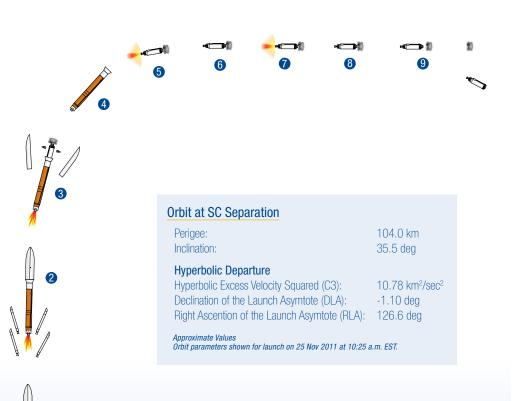
FLIGHT PROFILE | Liftoff to Spacecraft Separation
