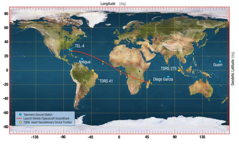
**1** = MECO (0:04:07.8) | **2** = SECO-1 (0:20:32.3) | **3** = 1st Restart— 2nd Stage (0:28:22.5) | **4** = SECO-2 (0:31:30.8) | **5** = WGS-6 Separation (0:40:37.5)
